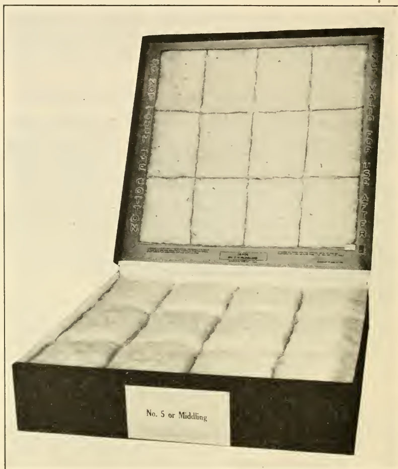
FIGURE 1.- Practical form of the universal standards for the grade of Middling White cotton. A photograph is shown inserted in the cover of the box to verify the preparation of the cotton and the position of the leaf. At the bottom of the photograph appears the seal of the Department of Agriculture and the certificate and signature of the Secretary of Agriculture. Standards for the other grades and colors are represented in the same manner.
